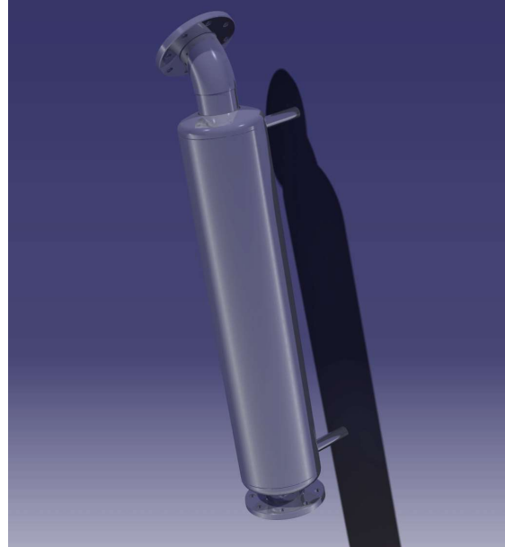
Fig. 8.14 Condenser, back view
