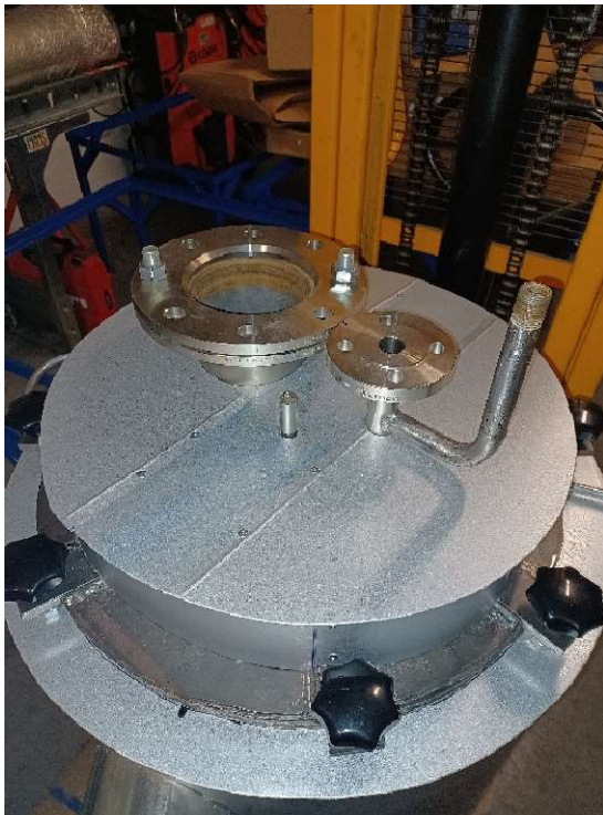
Fig. 8.25 Detail of the removable reactor cover
