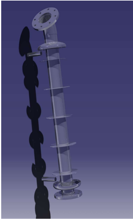
Fig. 8.15 Screens in the coolant circuit in the condenser, front view
