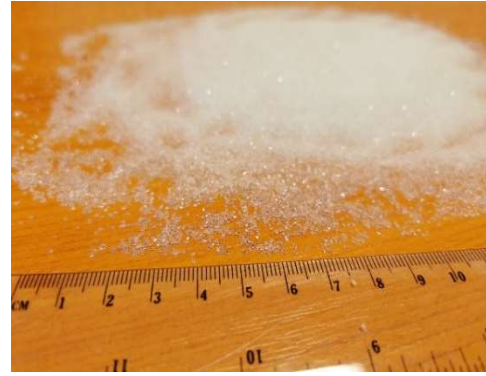
Fig. 6.23 Detail of the crushed glass
