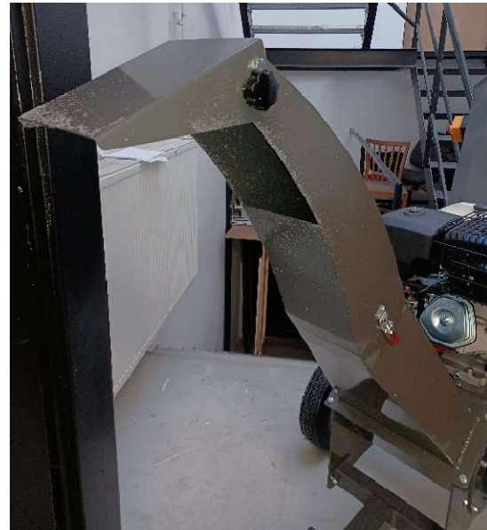
Fig. 8.30 Hopper for crushed material from the crusher
