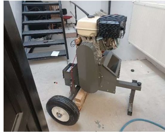
Fig. 8.28 Disassembled crusher after blade adjustment
