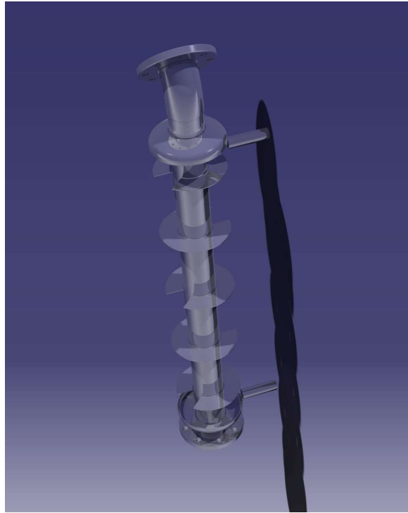
Fig. 8.16 Screens in the coolant circuit in the condenser, back view
