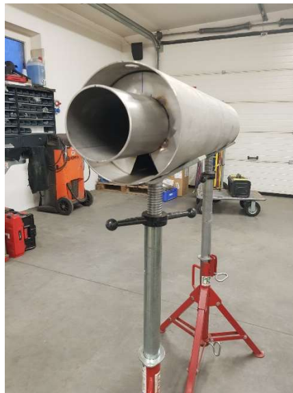
Fig. 8.18 View of the condenser prior to welding of the cooling circuit bottoms
