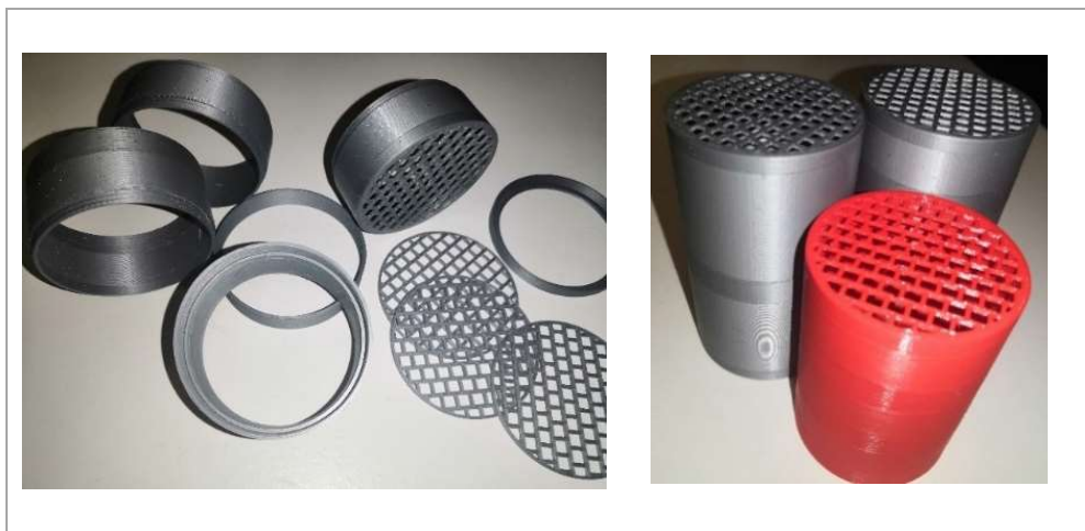
Fig. 6.31 Real view of the test cartridges – 3D printing
