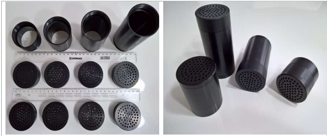
Fig. 6.29 Test cartridges – CNC machining
