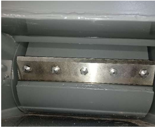
Fig. 8.27 Adjustable blades of the crusher
