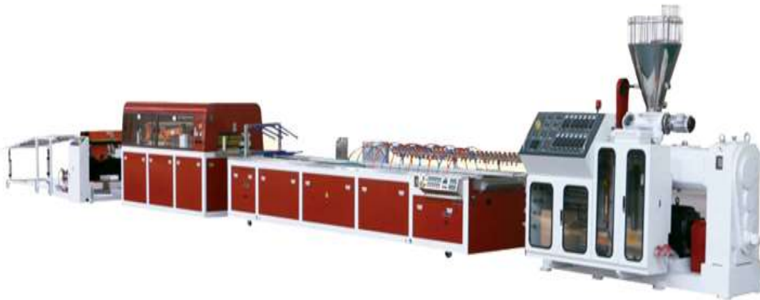
Fig. 7.4 Line for the production of wood-plastic boards ( www.res.cloudinary.com )
