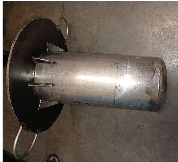
Fig. 8.23 Pyrolysis chamber pulled out of the reactor
