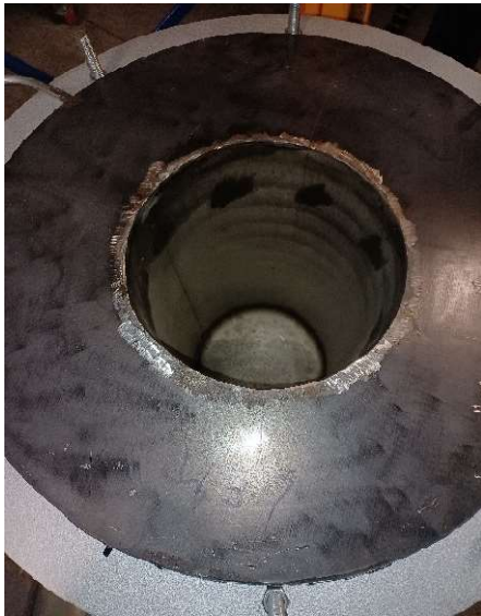
Fig. 8.22 View of the pyrolysis chamber of the reactor
