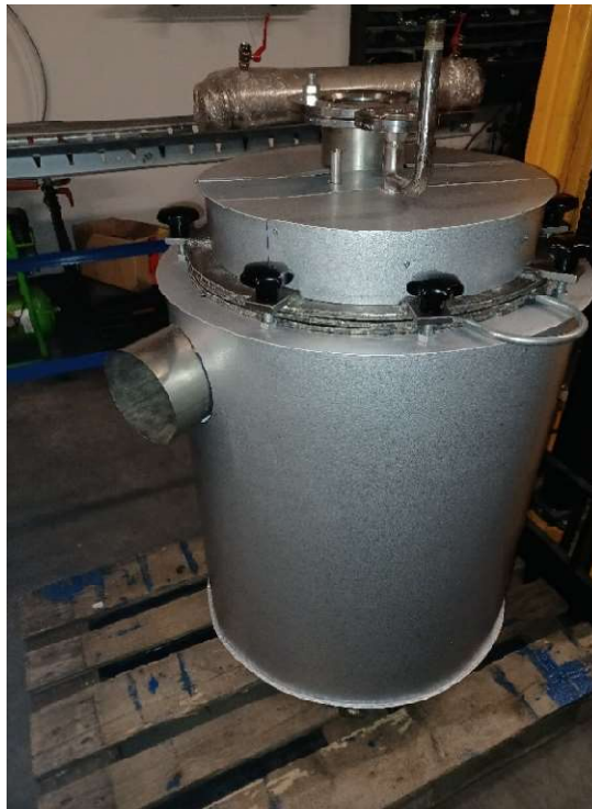
Fig. 8.26 Completed pyrolysis reactor without condenser
