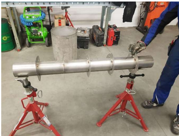
Fig. 8.17 View of the welded screens in the coolant circuit in the condenser
