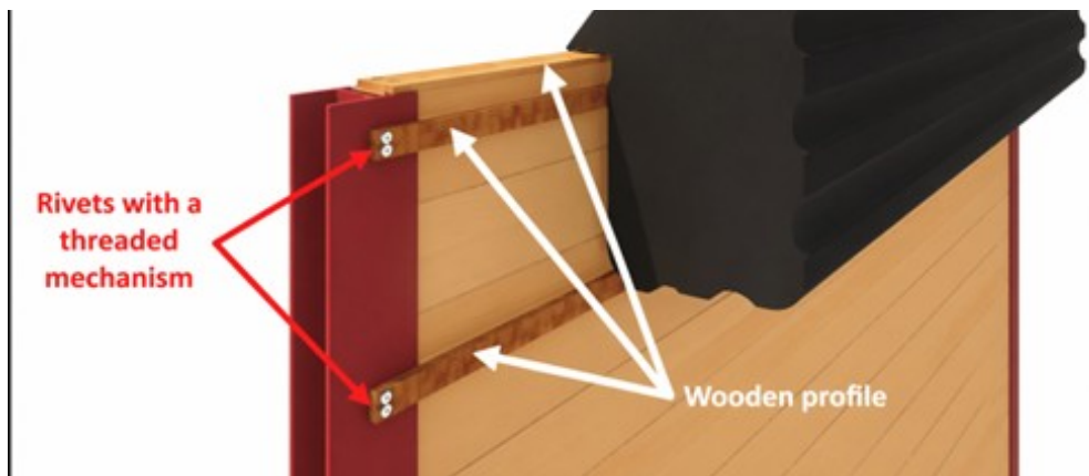
Fig. 3.10 View of the installed noise absorber on the noise barrier with mounting profiles
