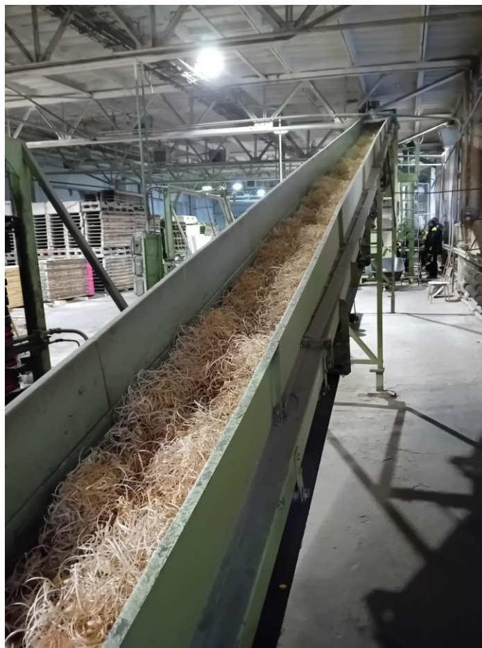
Fig. 5.3 Wood wool fed into the mixing drum
