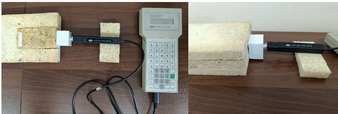
Fig. 2.22 Measurement of the thermal conductivity coefficient with the ISOMET 2114 instrument
