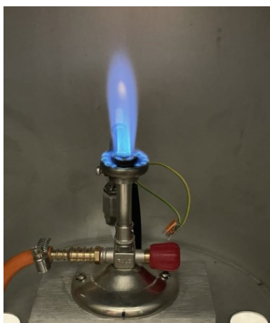
Fig. 4.12 Combustion of pyrolysis gas in the afterburner chamber
