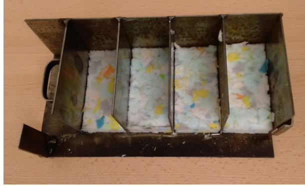
Fig. 2.9 Removing finished samples from the mould
