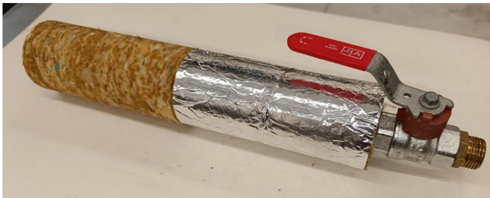
Fig. 2.24 Moulded part of pipe thermal insulation (without film / with aluminum film)
