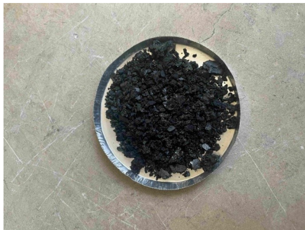
Fig. 4.14 Solid residue after pyrolysis of car seat covers
