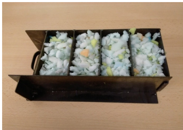
Fig. 2.7 Filling the mould with material
