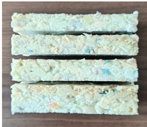
Fig. 2.11 Dependence of sample height (and thus density) on the magnitude of the loading pressure
