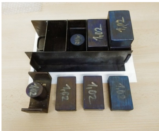
Fig. 2.6 Mould and weights for the production of experimental samples
