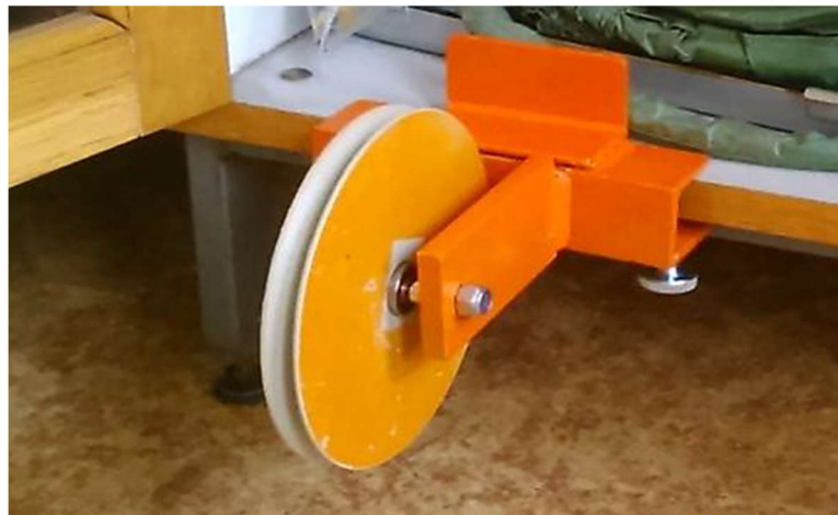
Fig. 89 End point of the cable travel path for driving antenna displacement
