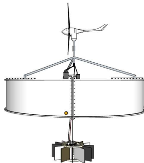
Fig. 169 3D view of a float device with a wind dynamo [120]
