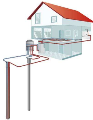
Fig. 67 Soil/water heat pump [84]
