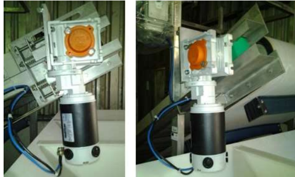
Fig. 222 Real views of the TRANSTECNO ECMP070/056/030 U electric motor [123]
