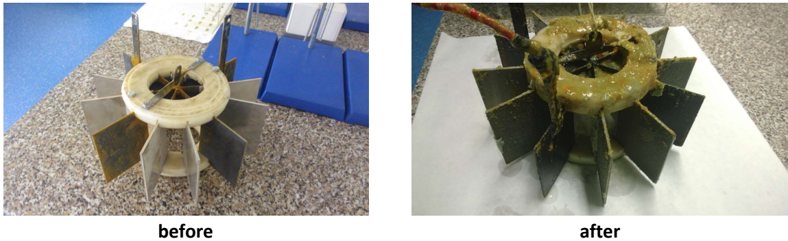
Fig. 187 Smallest star electrode before and after electro flotation applications in the laboratory [110]
