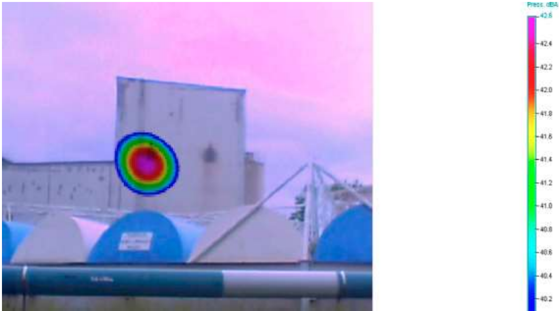
Fig. 247 Noise emissions of the visualized object across the frequency band (150 - 13 kHz) - measurement No. 4
