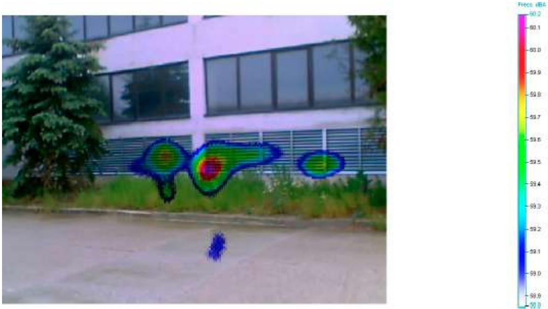
Fig. 243 Noise emissions of the visualized object in the 1500 - 2500 Hz frequency band - measurement No. 2
