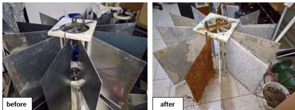
Fig. 192 Largest star electrode before and after electro flotation applications on the recreation area of the CP - Nad Jazerom in Košice [110]
