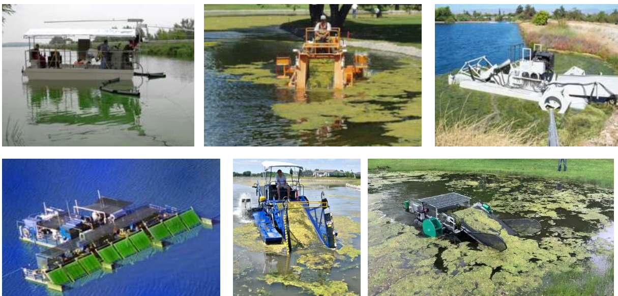
Fig. 145 Types of vessels for the separation of biomass particles from the surface of the water surface
