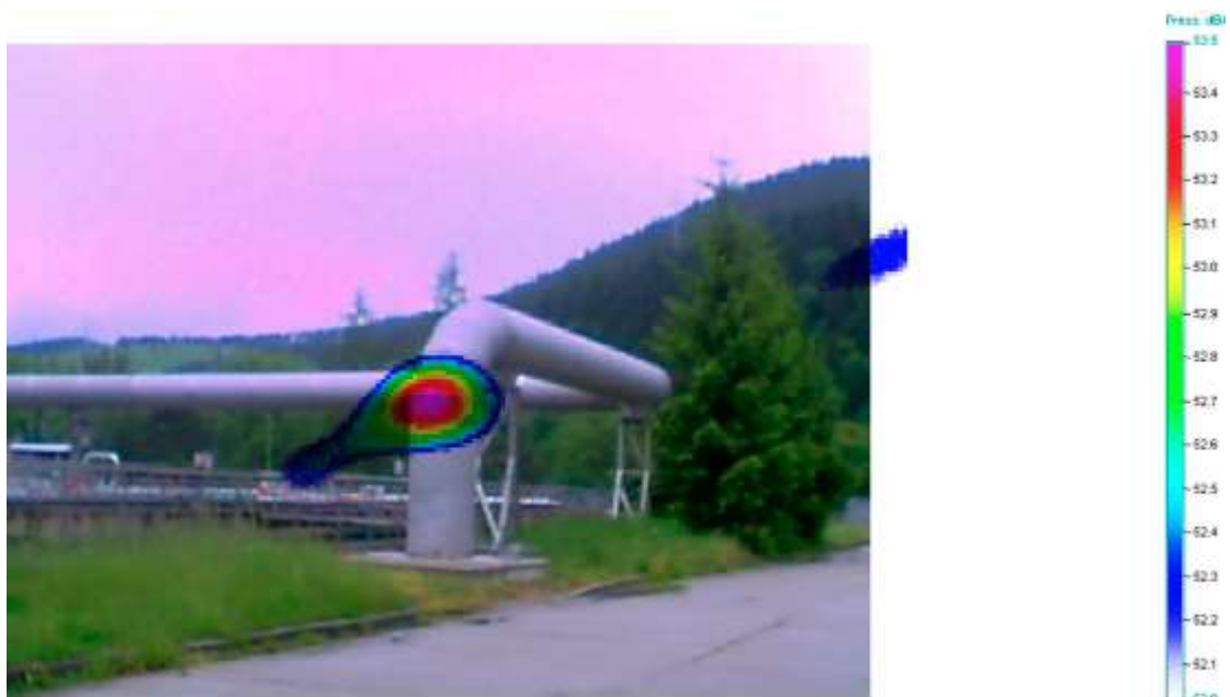
Fig. 237 Noise emissions of the visualized object across the frequency band (150 - 13 kHz)— measurement No. 1
