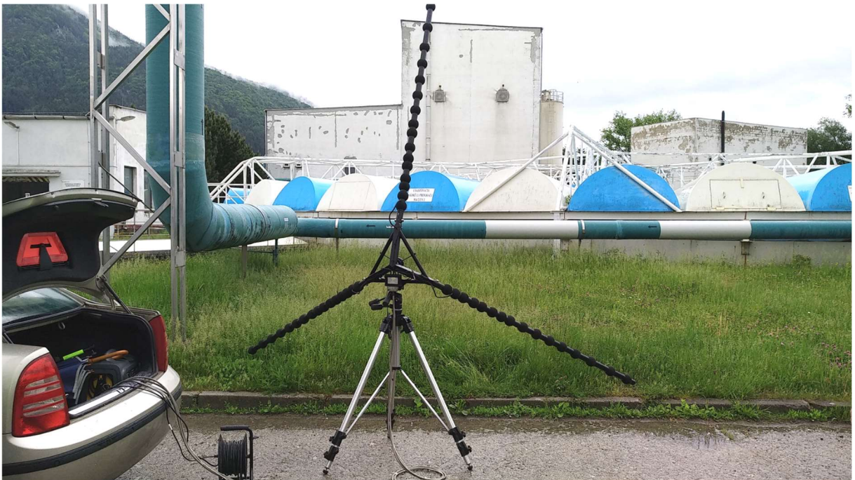
Fig. 246 View of the installed acoustic camera - measurement No. 4.
