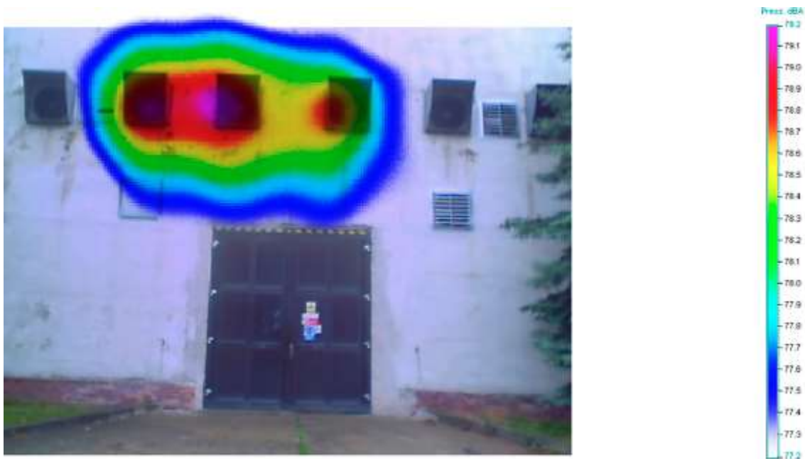
Fig. 244 Noise emissions of the visualized object across the frequency band (150 – 13 kHz) - measurement No. 3
